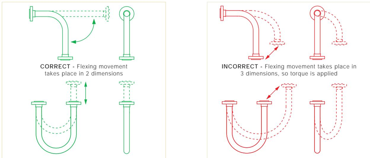
Both Corroflon and Bioflex hose have good resistance to a small level of torque, much better resistance than rubber or SS hose types, but it is still the best practice to take whatever steps are necessary to eliminate torque. If in doubt, consult Aflex Hose.
