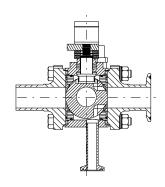
The **Closed Position** allows condensate to flow past the ball purge holes during normal operation. Condensate flows past the purge holes in the ball and out the side port of the valve to the steam trap, allowing the body cavity to remain hot. The point-ofuse, or sampling connection, is isolated by the surface of the ball without the purge holes.
