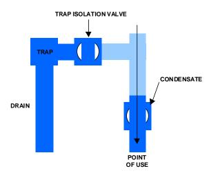
When steam is in use, the point of use valve becomes cold from condensate buildup. Ideal conditions exist for bacterial growth.
