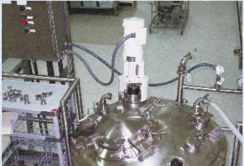
*(Above) A 2500 gallon pharmaceutical blending tank is mixed with a sanitary design SHARPE mixer. The dry-running mechanical seal operates without the use of external lubrication. All surfaces exposed to the product were mechanically polished to a 15 Ra finish and electropolished for optimum sterilization.*
