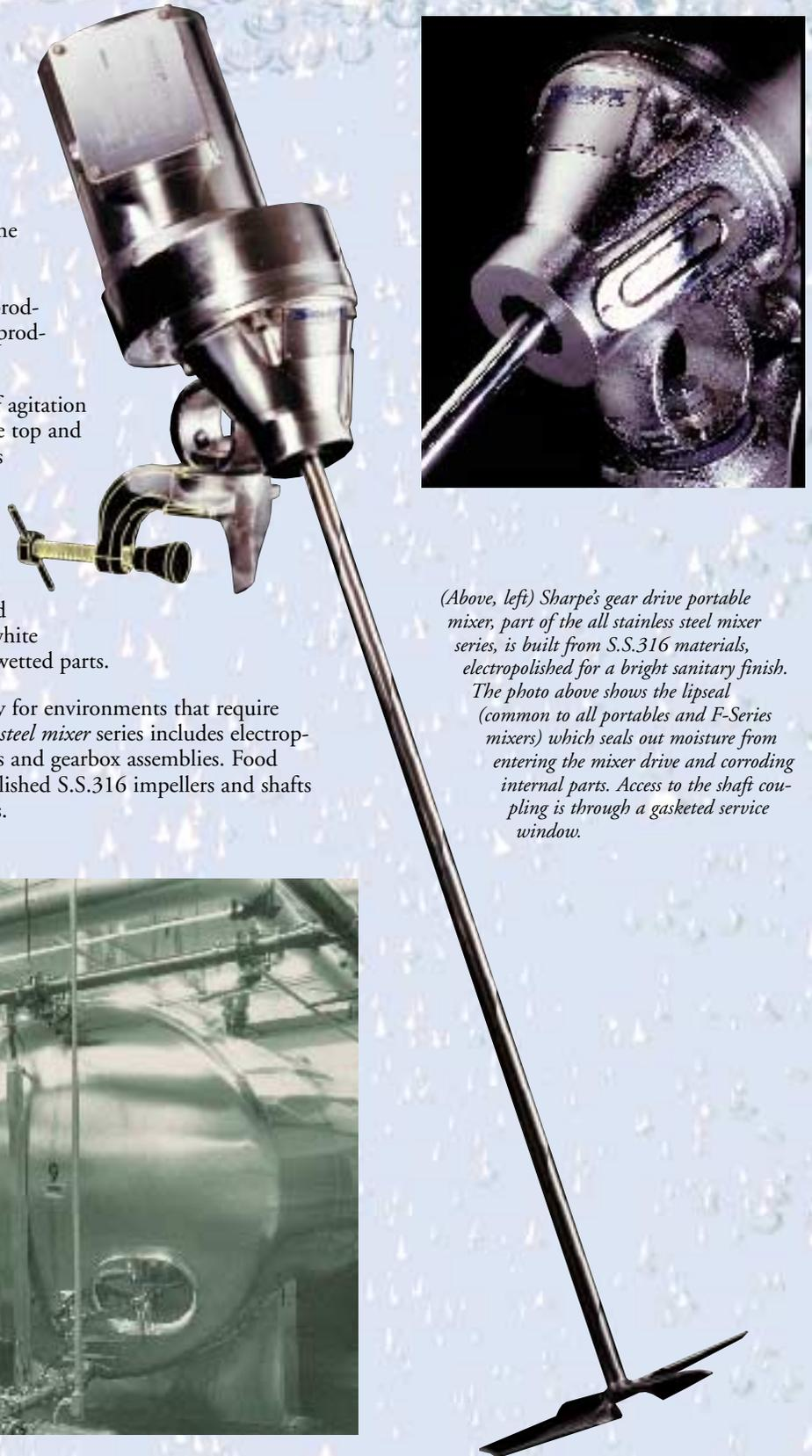
*(Above, left) Sharpe's gear drive portable mixer, part of the all stainless steel mixer series, is built from S.S.316 materials, electropolished for a bright sanitary finish. The photo above shows the lip seal (common to all portables and F-Series mixers) which seals out moisture from entering the mixer drive and corroding internal parts. Access to the shaft coupling is through a gasketed service window.*
