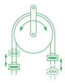
The Fourth Rule is that the hose must not be subjected to torque, either during connection, or as a result of the flexing cycle.
