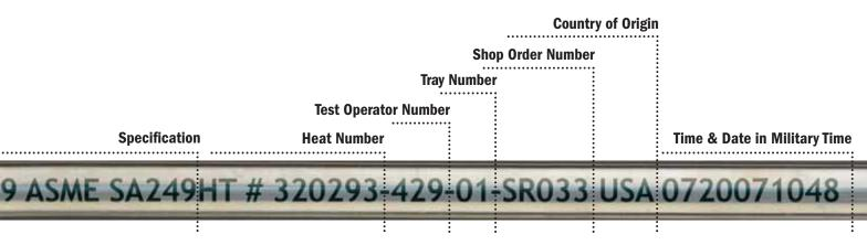
(ABOVE) Line marking is an important key to maintaining quality control and traceability. Complete product description, specifications, manufacturing and testing information are included.
