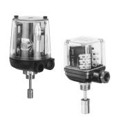
The GEMÜ 1214 and 1232 electrical position indicators have one or two proximity switches for end position feedback which are mechanically adjustable.
