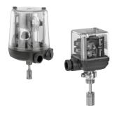
The GEMÜ 1211 and 1231 electrical position indicators have one or two proximity switches for end position feedback which are mechanically adjustable. The devices are suitable for installation in Ex-proof applications acc. to ATEX. GEMÜ 1211 is suitable for mounting to linear actuators with a max. stroke of 70 mm. GEMÜ 1231 is suitable for mounting to linear actuators with a max. stroke of 20 mm.
