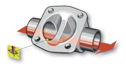
In the pharmaceutical and biotechnological industries and other sensitive industrial sectors the drainability and cleanability of plant plays an important role. Very often plants are cleaned and sterilised after every production process. The objective is to keep the residue as low as possible in order to optimise the sterilisation and cleaning processes of plant and piping systems.
