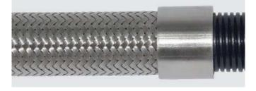
The braid supports the PTFE liner tube against internal pressure and protects against mechanical abuse. Often used in applications involving high temperatures and working pressures. High tensile 304 stainless steel wire is used to give maximum pressure resistance and external protection to the hose.
