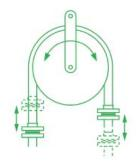
The Fourth Rule is that the hose must not be subjected to torque, either during connection, or as a result of the flexing cycle.
