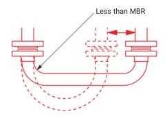
INCORRECT - Weight of hose is at 90° to Axis of End Fittings
