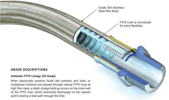
Antistatic PTFE includes a small quantity of a special carbon black which ensures safe static charge dissipation, in accordance with International Standards.
