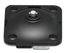
The Saunders® SR diaphragm features the Saunders® bayonet type compressor attachment which allows the diaphragm to float freely relative to compressor to avoid point loading of the TFM at the stud. The bayonet fit also facilitates easy error free engagement of diaphragm and compressor.
