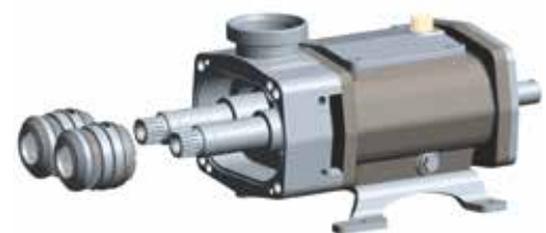
4. Exchange of mechanical seals
