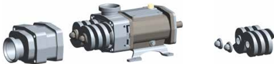
1. Removal of pump casing and cover
