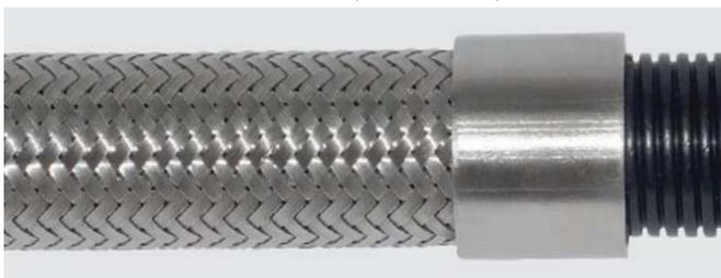
The braid supports the PTFE liner tube against internal pressure and protects against mechanical abuse. Often used in applications involving high temperatures and working pressures. High tensile 304 stainless steel wire is used to give maximum pressure resistance and external protection to the hose.
